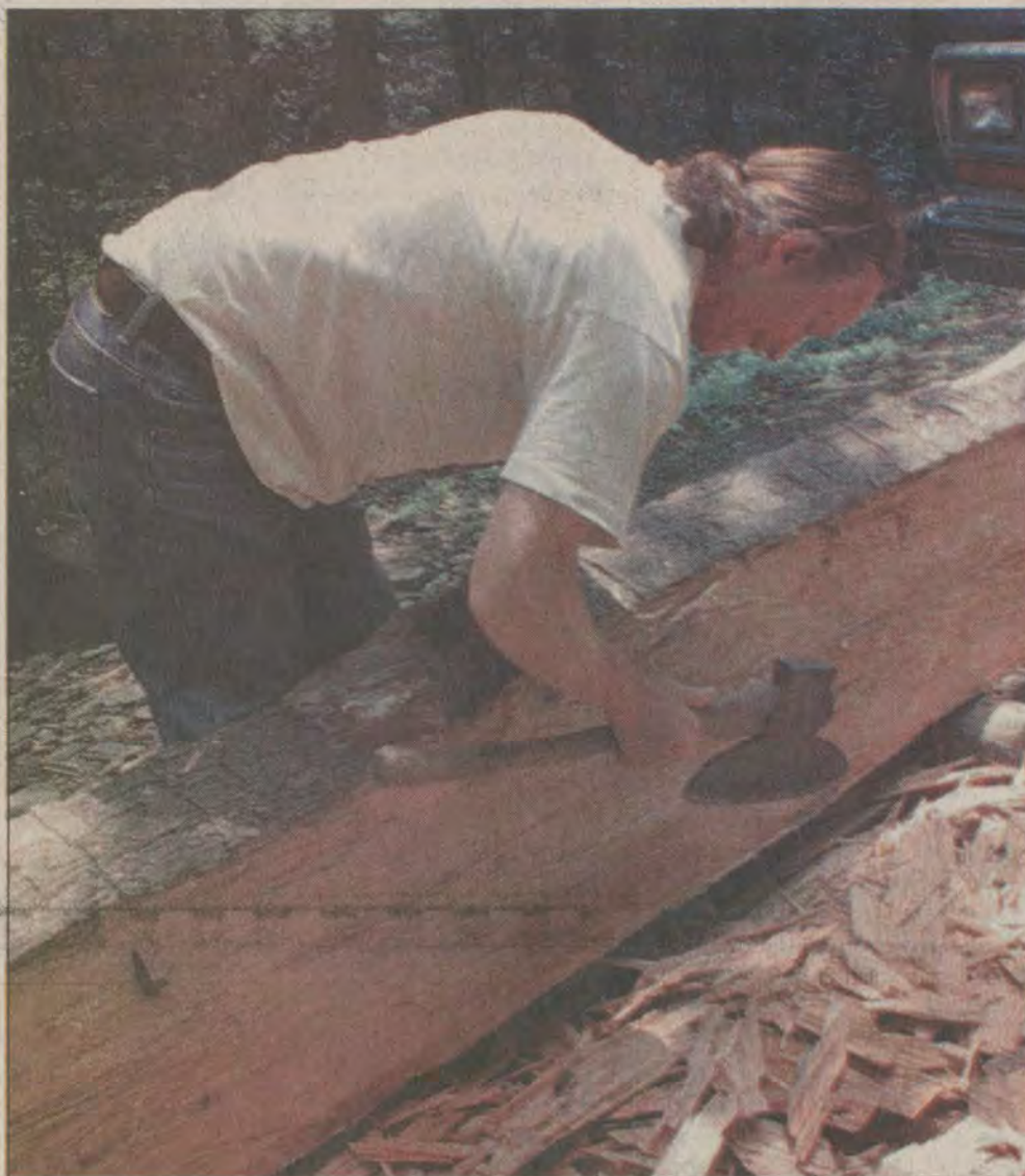
The craftsman hewing a slab of timber that will later become a mantle.
