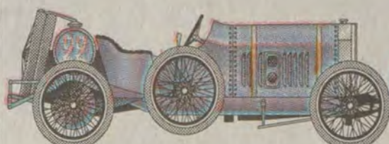
1912, 7.6 liter G.P. Peugeot Won first place in the French Grand Prix with an average speed of 68.45 mph (110 kmph).
