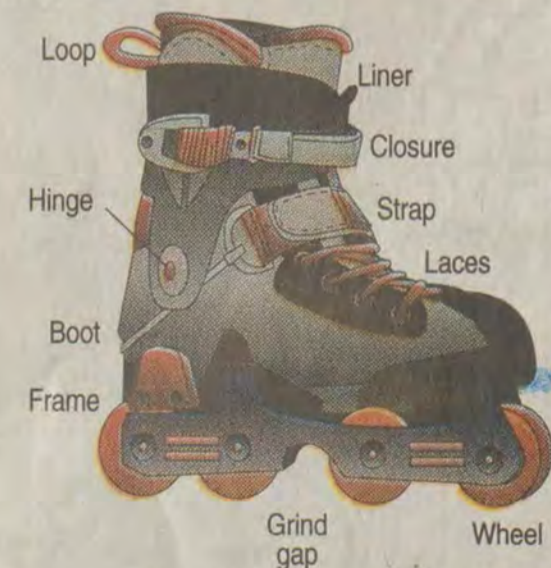
Aggressive in-line skates are sturdy and heavy to protect the feet. Small, hard wheels provide maximum maneuverability.
