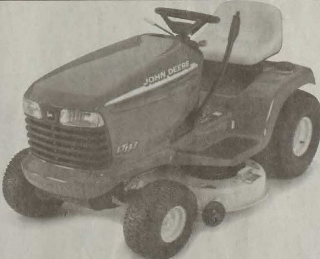
LT133 Lawn Tractor • 13-hp • 38-inch mowing deck • 5-speed shift-on-the-go transmission
