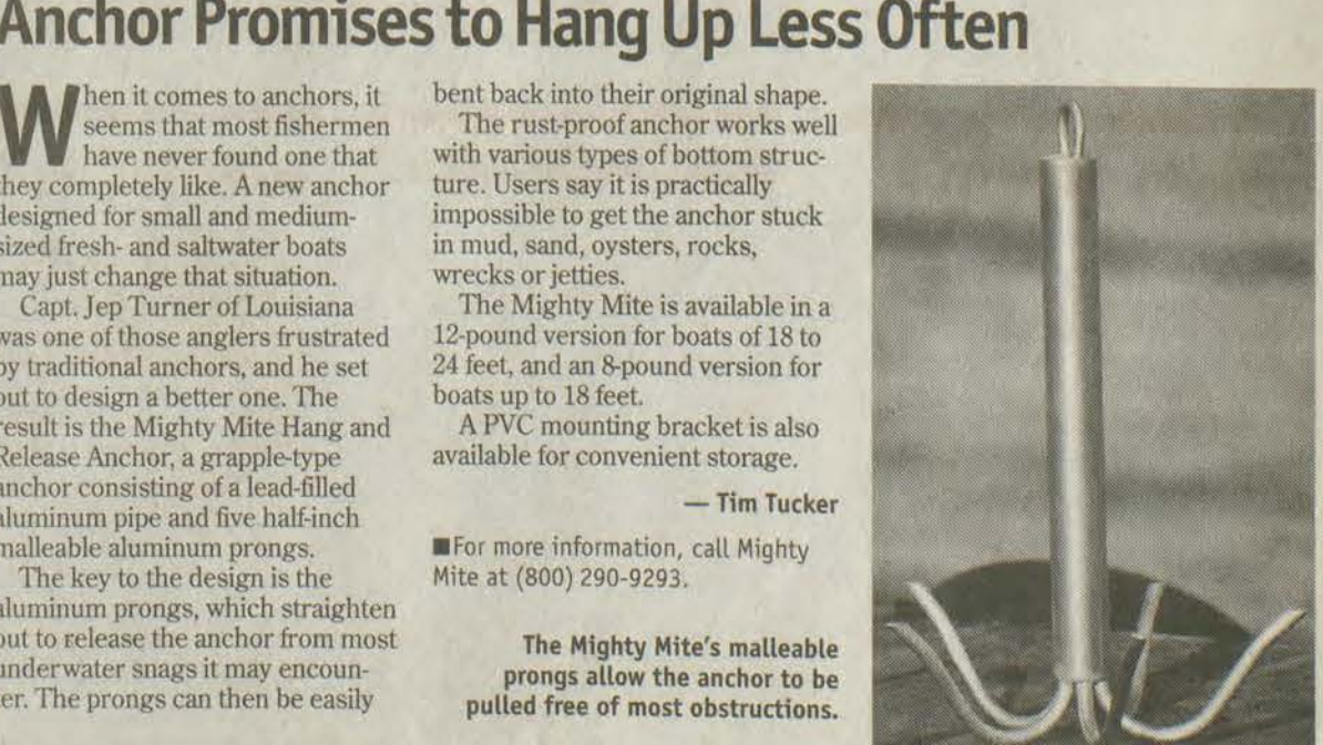
The Mighty Mite's malleable prongs allow the anchor to be pulled free of most obstructions.
