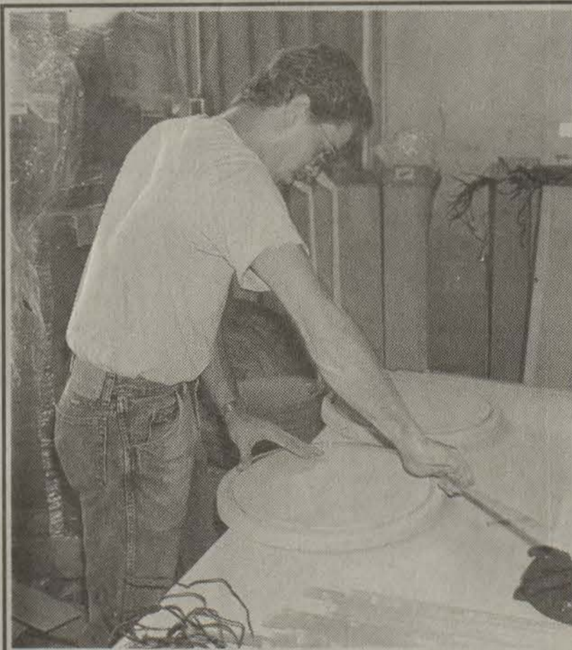
Phil Conrad of Prestonsburg attaches a ring of lights to a concrete stepping stone which RND produces. The stones can be arranged to provide lighted walkways around homes or in public areas.
