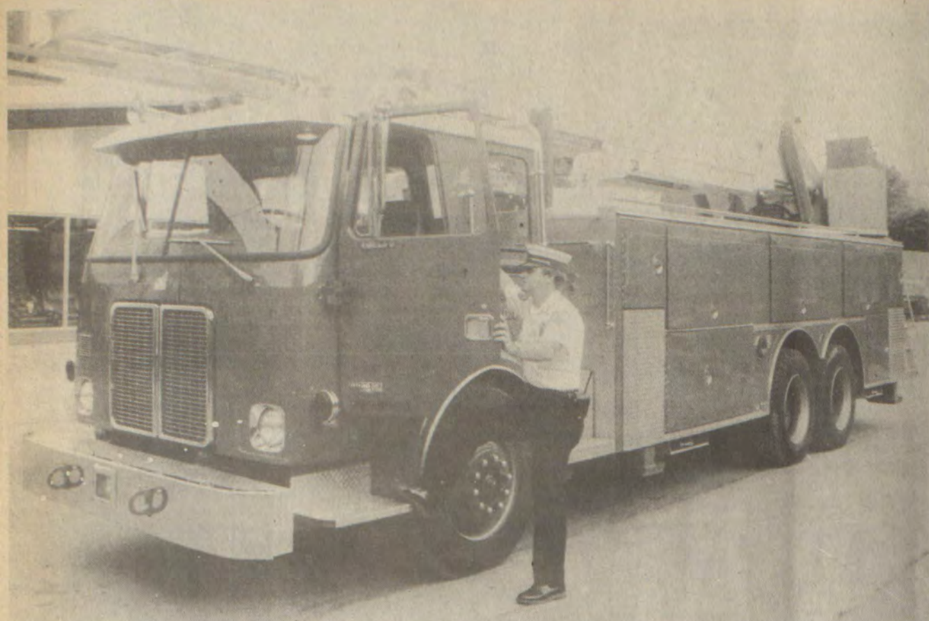
PRESTONSBURG FIREFIGHTERS will practice until they can set up the city's new ladder truck in 90 seconds, Capt. Larry Adams, pictured, said last week, shortly after he and Capt. Paul Burke drove the $179,000 truck here from Nebraska. The new unit has a 104-foot ladder with a telescoping water hose, which will enable fire crews to reach the city's tallest structures and perhaps will lower insurance rates as well.
