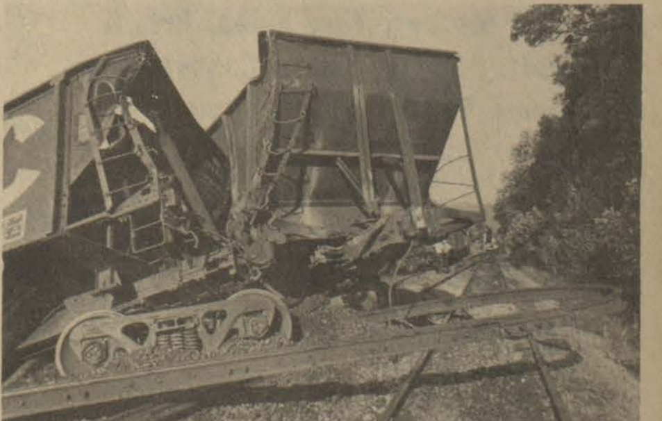
Jumbled cars and bowed rail pictured following the derailment Saturday of nine, loaded C. & O. coal gondolas at Auxier. The mishap apparently resulted after an axle broke on one of the cars with the actual derailment occurring after the crippled "gon" had been dragged approximately one-half mile along the track.
