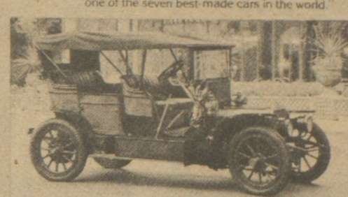
The 1906 chain-driven Torpedo, powered by an advanced four-cylinder, 12 horsepower engine.
