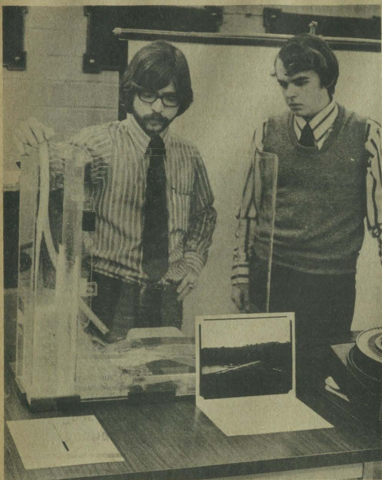
RESERVOIR WATER PRESSURE DEMONSTRATED. —Dean Perry, Prestonsburg (left), and Harry Sterling, Ashland, demonstrate an exhibit they constructed for Engineering Week open house at the University of Kentucky. Both students are seniors, majoring in civil engineering. The exhibit shows how water pressure in a reservoir opens a gate to control a stream's level of flow.
