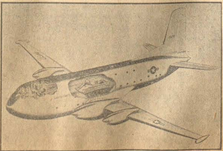
TANKS VIA AIR EXPRESS—This is an artist's conception of the turbo-prop powered YC-124B heavy transport the Douglas Aircraft Company has contracted to build for the Air Force. Capable of carrying a light army tank, the 22,000-horsepower sky giant is scheduled to roll off assembly lines at Long Beach, Calif., in the spring of 1952. In the cut-away view of the cabin, note the bunks built to accommodate crew members.
