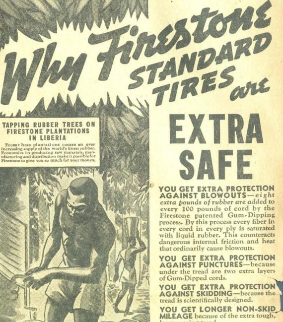
YOU GET EXTRA PROTECTION AGAINST BLOWOUTS—eight extra pounds of rubber are added to every 100 pounds of cord by the Firestone patented Gum-Dipping process. By this process every fiber in every cord in every ply is saturated with liquid rubber. This counteracts dangerous internal friction and heat
