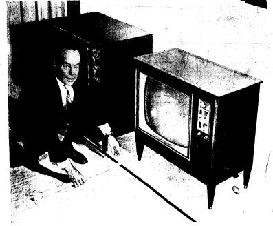
Motorola offers a choice in color television receivers for 1964. The set on the left uses the conventional 21-inch\* round tube, while the set at the right uses the new Motorola-developed 23-inch\* rectangular tube, allowing a reduction in the height, length and depth of the set. Demonstrating the five inch difference in the depth of the sets is Edward R. Taylor, Motorola's Executive Vice President in charge of Consumer Products.
