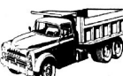
Heavy-duty Dodge Power Giant tenders deliver up to 232 hp., haul as much as 11,000 lbs. more payload. From 26,000 lbs. to 46,000 lbs. G.V.W., to 65,000 lbs. G.C.W. Three models, eight wheelbases.
