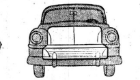
THE OLD WAY—Old-type construction limits interior space, so seats must be made narrower.
