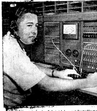
Guided by electronic "eyes and ears", the test deskman spots line troubles at once and gets repairs there quickly, often before service is actually interrupted.
