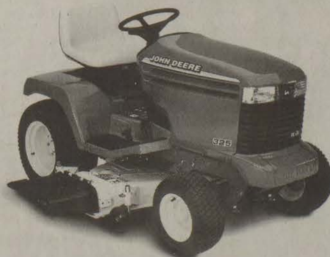
The 325 with 48" cutting deck and a high-torque 17-hp engine.
