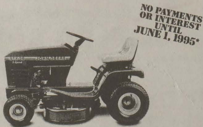
The STX38 with 38" cutting deck and a 12.5-hp engine.
