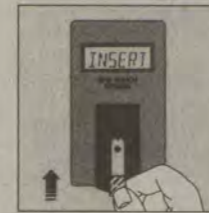
Press power, insert strip. (The last test result appears.)
