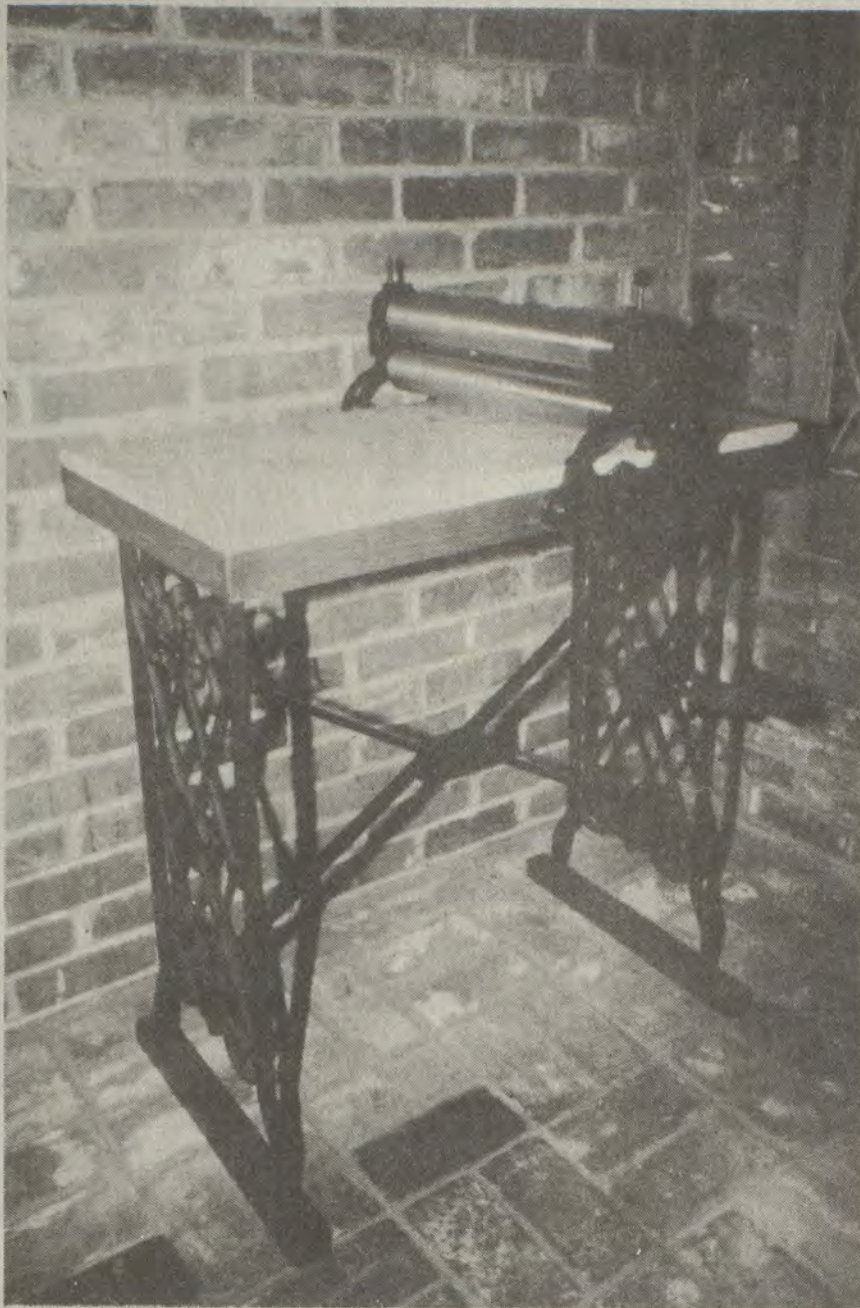
WRIGHT WALLER'S NEW PATENT BISCUIT MACHINE is made of two stainless steel rollers mounted on a cast marble top. It is presently on sale at the antique mall—Todd Square in Lexington.
