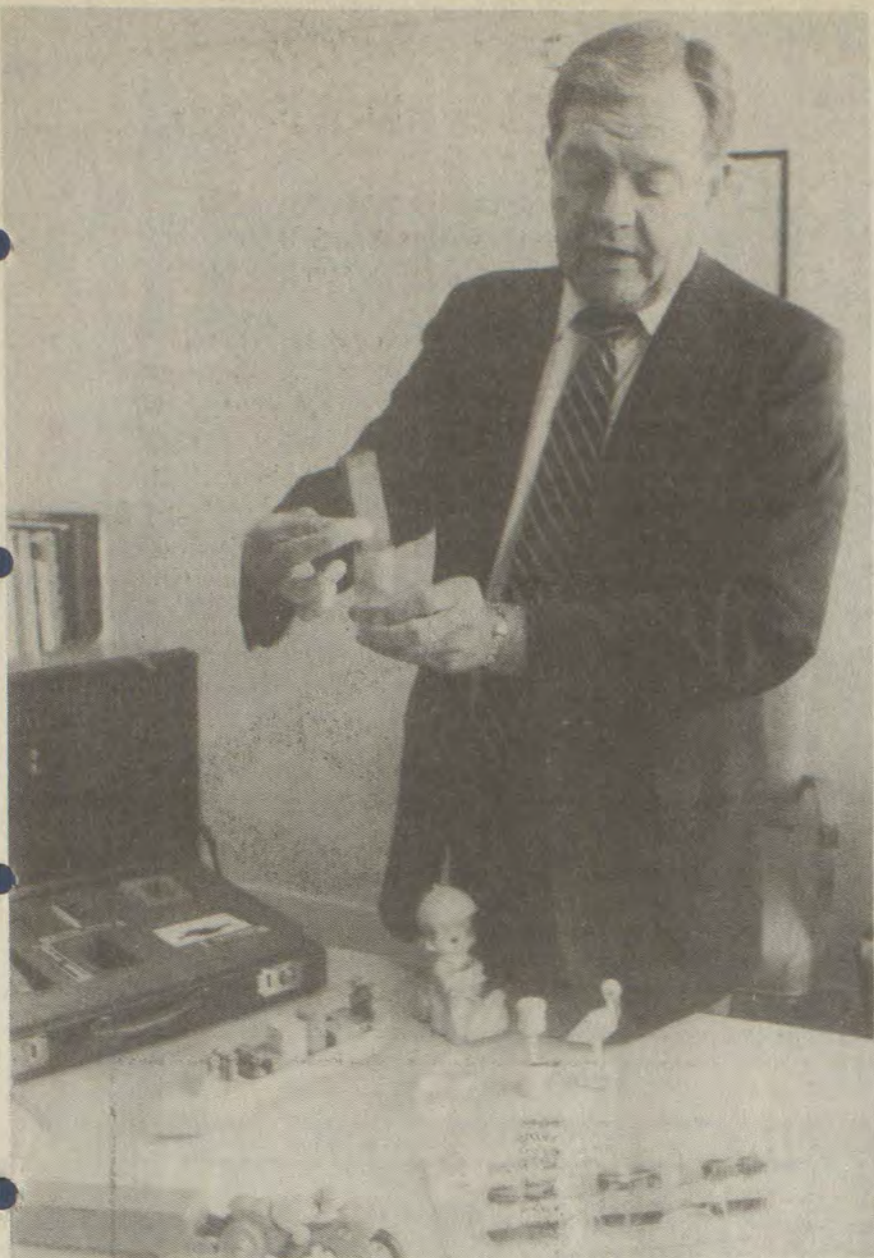
E.P. CONYERS demonstrates a "small parts" test for toys. Any toy or part of a toy that fits into the cylinder fails the test. The inspection kit is used by Department for Health Services inspectors. All of the toys pictured have failed various safety tests.
