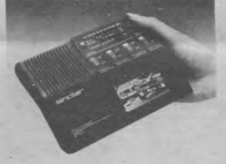
Measuring just 6 x 4 x 1 inches, this prototype represents the pocket television invented by Sinclair Research Ltd. of Cambridge, England. The prototype leatures a 3-inch diagonal black-and-white flat screen and incorporates an FM radio.
