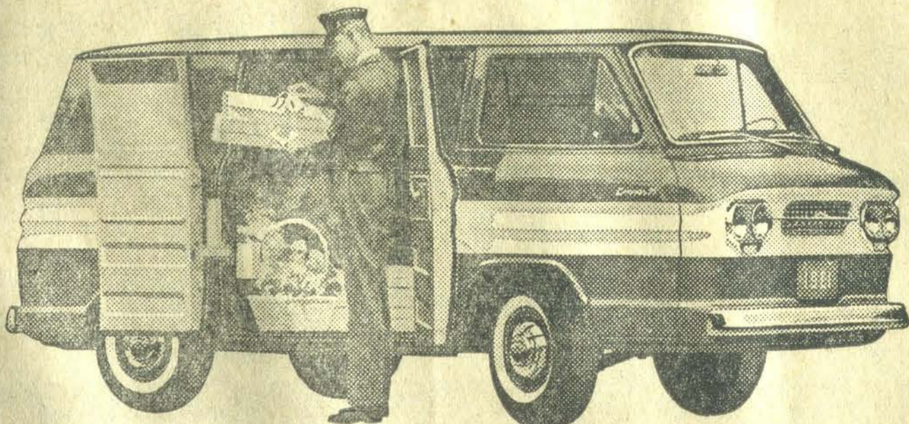
CORVAIR—Side doors open a full 49" wide. Loading height is a low 14" H1E1
