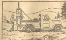
Mobile drill, mounted on the 'Jeep' Truck, is operated from the truck engine, through power take-off.
