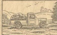
Hauling: The rugged 'Jeep' Truck carries a one ton payload... 63% of its curb weight! 6,000 lbs. G.V.W., 118 inch wheelbase.
