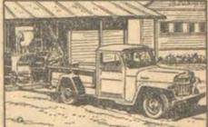
Belt power: With power take-off, it serves as a power unit for operating many types of belt-driven equipment.
