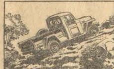
Extra traction of its 4-wheel drive takes the 'Jeep' Truck up 60% grades—through mud, snow, sand. It shifts into 2-wheel drive for highway travel.
