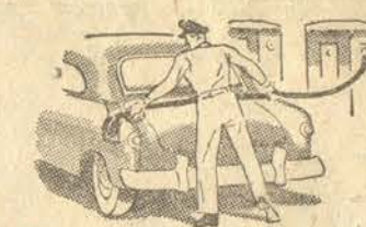
THE OLD WAY —Gas filler cap on fender... unhandy to reach from far side... unsightly.
