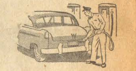
THE WILLYS WAY —Gas filler cap near center at rear... easy to reach from either side of car.
