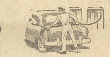
THE OLD WAY —Gas filler cap on fender... unhandy to reach from far side... unsightly.
