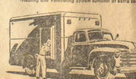
HEAVY-DUTY CAB-AND-CHASSIS with Refrigerator Body Model 6403—161-inch Wheelbase Maximum G.V.W. 16,000 lb.
