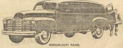
Model 3805—137-inch wheelbase, Maximum G.V.W. 6760 lb. Also available in light-duty Model 3105-116-inch wheelbase, Maximum G.V.W. 4600 lb.
