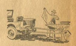
YOU GET POWER. The Universal "Jeep" provides three kinds of power; bulling power that operates tilling and harvesting equipment at tractor speeds of 21/2 to 7 mph; hauling power that can carry up to 1200 lbs, or tow a braked load of 21/2 tons on or off the road; portable power that furnishes up to 30 h.p. for operating all types of splineshaft or belt-driven farm machinery.
