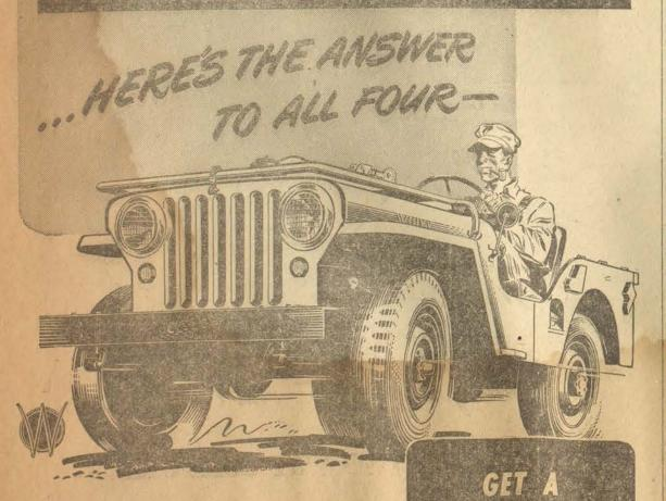
THE UNIVERSAL 'JEEP' is built to handle almost any kind of job. It has 4-wheel drive, with speeds as low as 21/2 mph, for tractor work, for heavy towing, for getting through mud and snow that stops ordinary vehicles. It has 2-wheel drive for hauling and towing at highway speeds. It has optional power take-off, with spline-shaft or pulley drive, to operate auxiliary equipment. Let us demonstrate this versatile vehicle and show you how it meets your needs,
