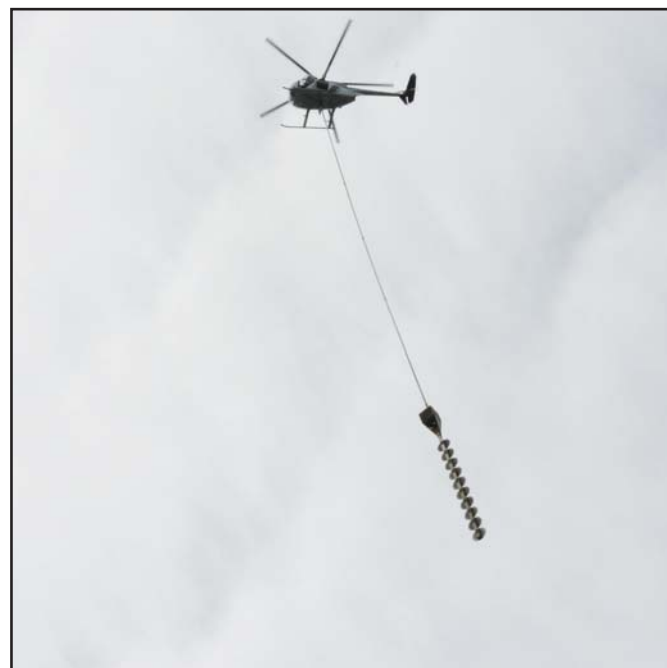
Appalachian Newspapers photos by Aaron K. Nelson One of North Carolina-based Aerial Solutions' air saws, piloted by Barbie Rise, takes to the skies over Thelma this week to clear right-of-ways for transmission lines in Johnson County. The saw was also recently used in Floyd County.
