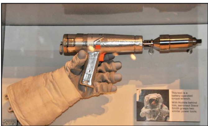
A battery-operated torque wrench and other types of tools used to service the Hubble Space Telescope are on display.
